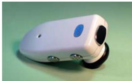
All hands-free profile features are supported and accessible via the Man-Machine-Interface (MMI). A three button design is used to allow easy access to the volume control and phone answer/end buttons. An incoming call will ring through to the headset and
