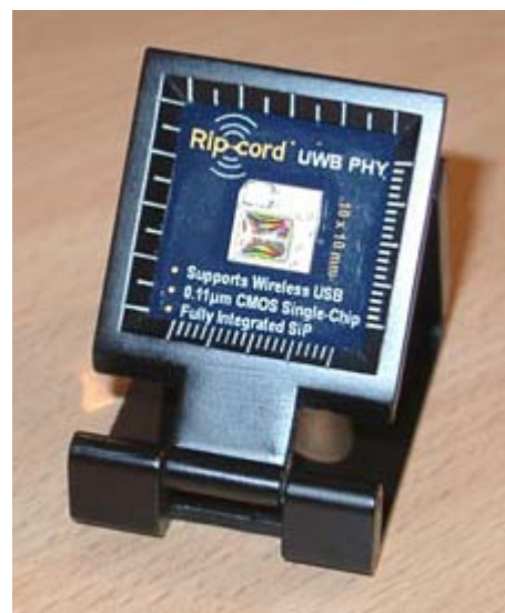
Staccato's Ripcord System-in-Package (SiP) module is comparable in size to current Bluetooth radios and contains all electronics and passive elements necessary for operation except the antenna.
