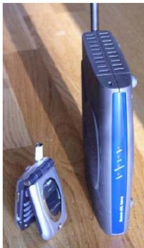
A couple of IVT's example reference designs: a clamshell GSM phone with CTP-enabled class 1 Bluetooth, and a CTP-enabled ADSL access point - also class 1
