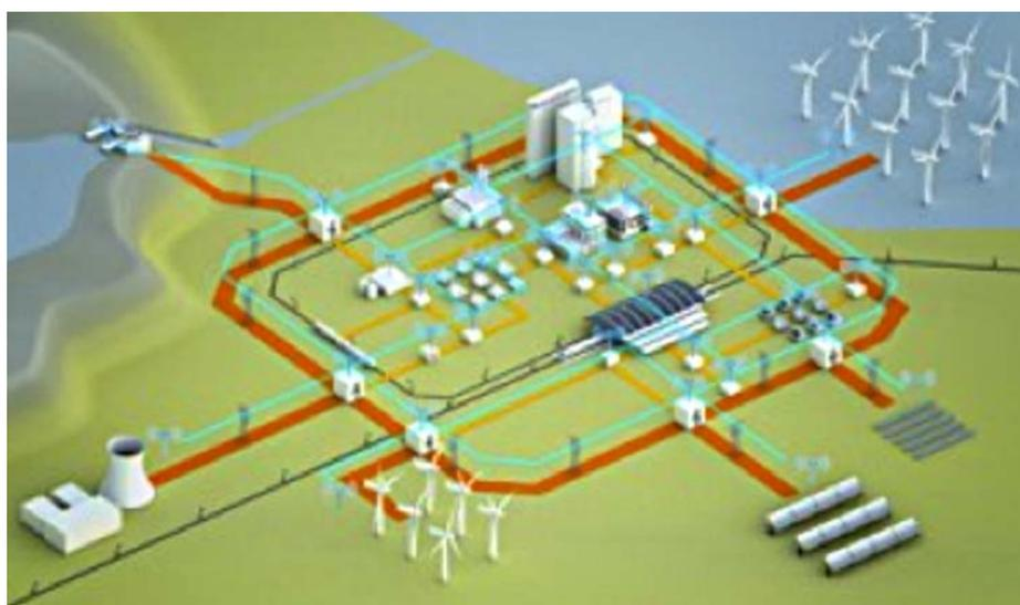
*A smart grid ensures that renewable energy sources can be better integrated into the grid thanks to bidirectional flow of energy (orange line) and a bidirectional flow of communication data (blue line).*
